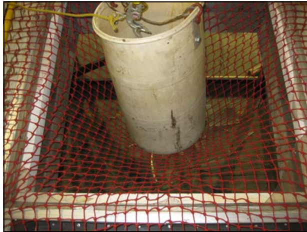
SKYNET over shattered skylight after drop
